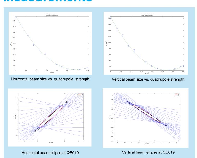
**Top:** Measurements of the square of the beam sizes  $\sigma_x^2$  and  $\sigma_y^2$  for the 6 GeV case. An error of  $\Delta(\sigma_x) = 0.4$  mm and  $\Delta(\sigma_y) = 0.2$  mm for the fitting of the profiles was assumed.
