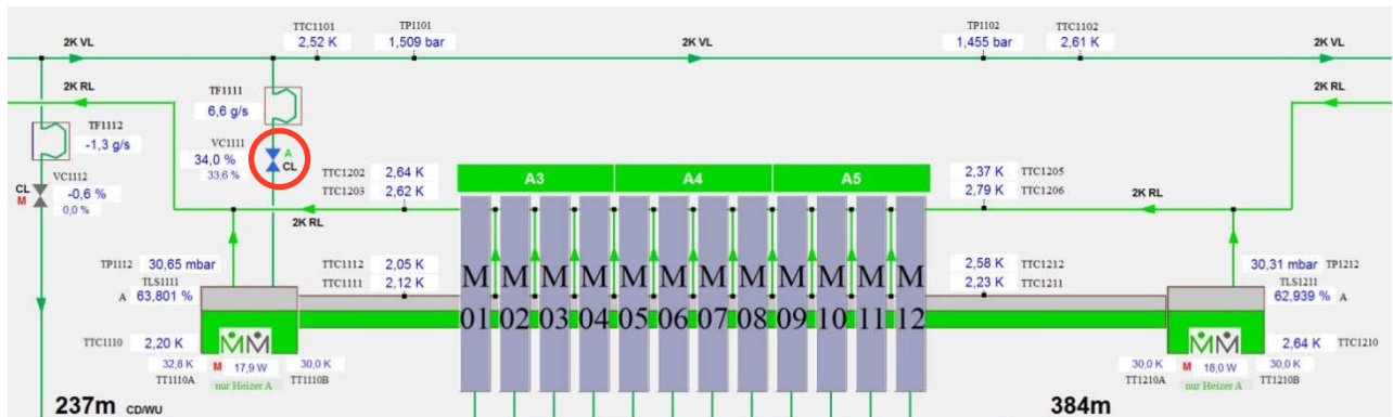
Figure 2: A cryo string in the XFEL consists of of twelve cryo modules. The main control loop is configured to keep the LHe level constant by setting the JT valve accordingly.
