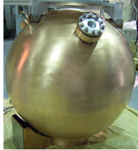
Figure 1: a left) Principle of spherical gas detector - b right ) 60cm prototype made of low activity Copper
