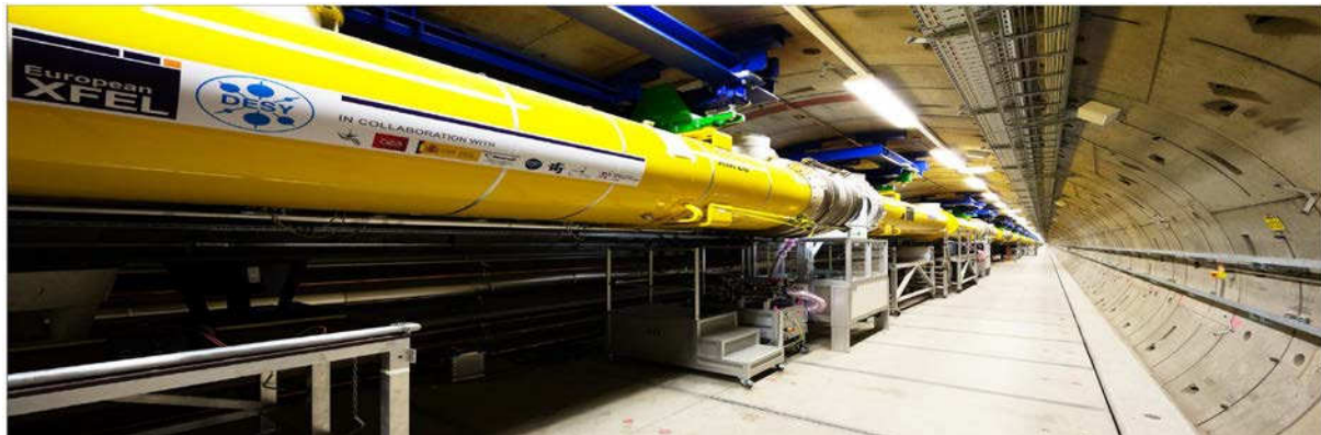
Figure 2. Cryomodules inside XFEL tunnel.
