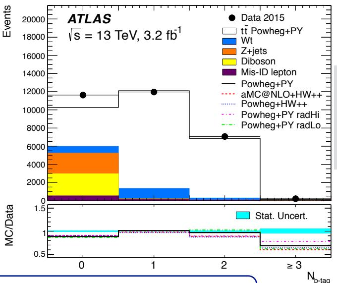
$$\sigma_{t\bar{t}} = 818 \pm 8_{\text{stat}} \pm 27_{\text{syst}} \pm 19_{\text{lumi}} \text{ pb}$$
