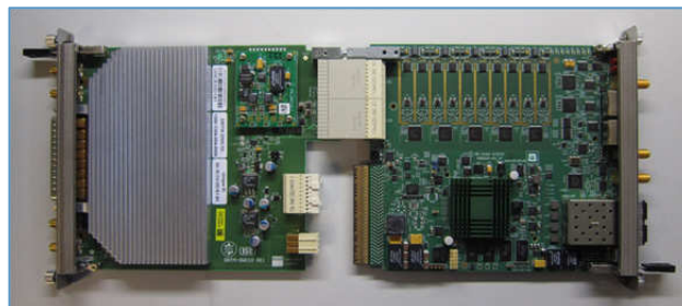
Figure 1: MicroTCA.4: Front-side AMC board (right), Rear-side RTM board (left).
