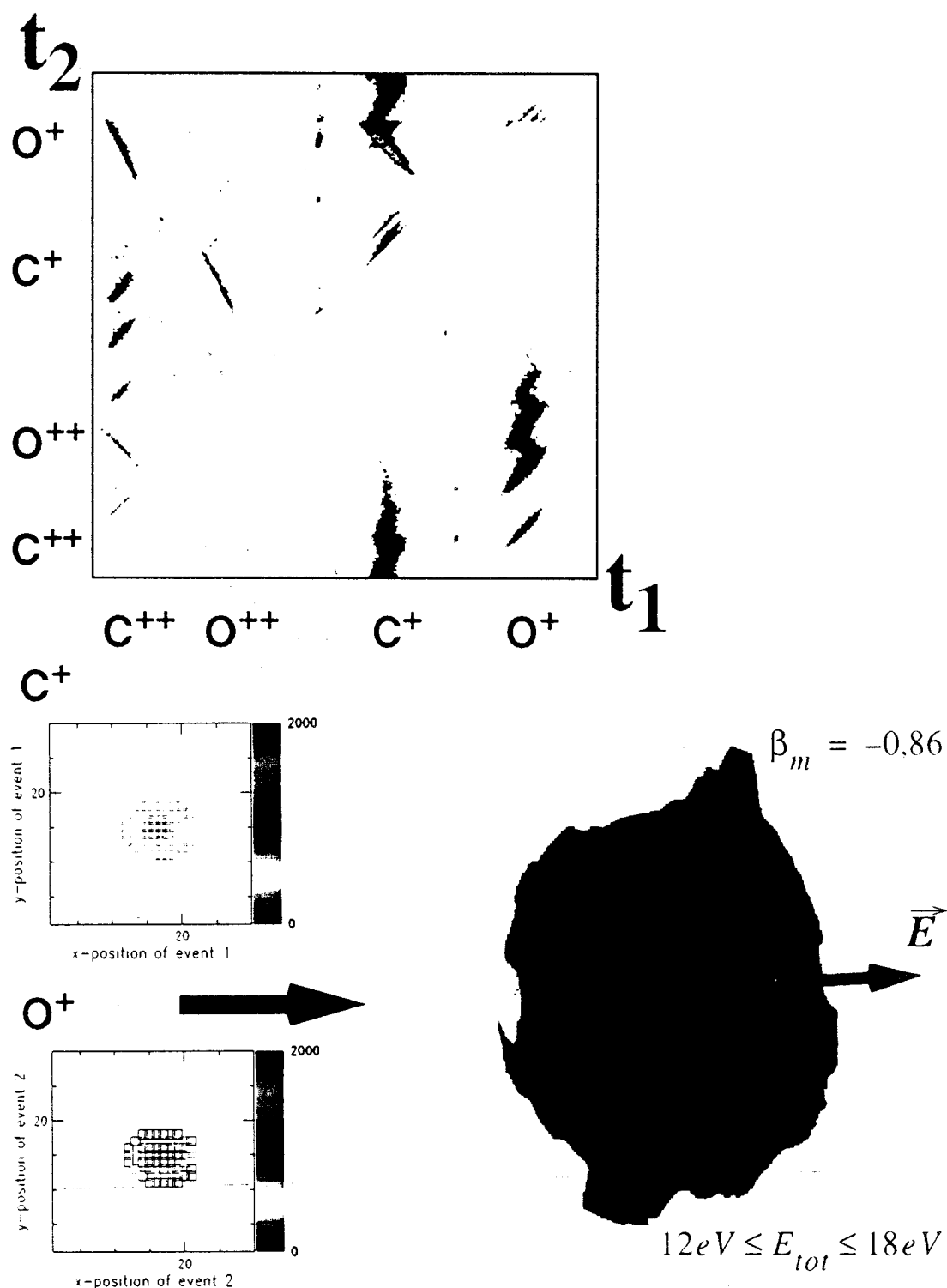
FIG. 2. Top: coincidence map of the flight time of the first and second detected ions. Lower left: position of the first and the second detected ions on the MCP, which correspond to C^+ and O^+ ions, respectively. Lower right: three-dimensional representation of the angular distribution for C^+ + O^+ ion pairs with total kinetic energies between 13 and 18 eV.
