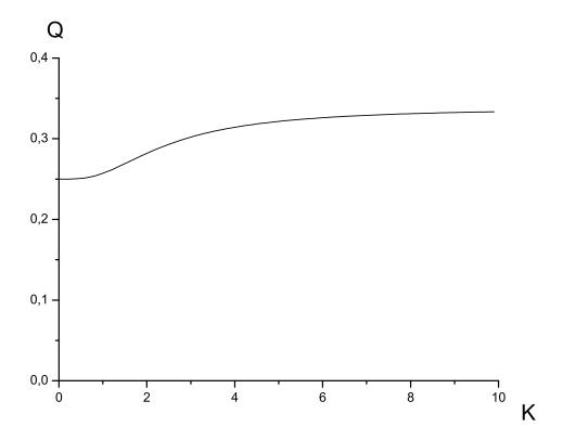
Fig. 1. Illustration of the behavior of the ratio Q(K) between the second harmonic field contribution due to the gradient of the density part of the source and the contribution due to the current part of the source.
