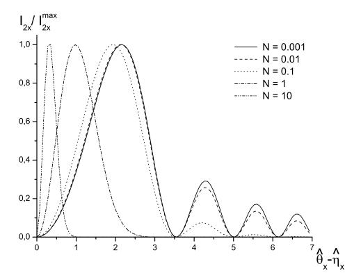
Fig. 2. Plot of the directivity diagram for the radiation intensity as a function of  $\hat{\theta}_x - \hat{\eta}_x$  at  $\hat{\theta}_y - \hat{\eta}_y = 0$  for the horizontal polarization component, for different values of N.
