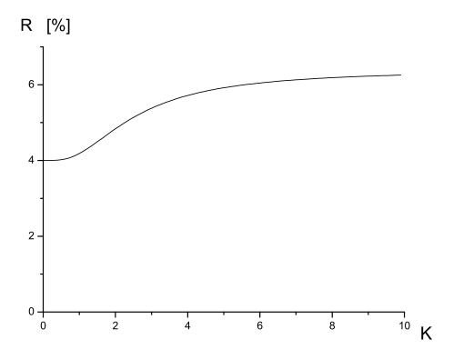
Fig. 6. Illustration of the behavior of the ratio between the second harmonic power due to the y vertical and the x horizontal polarization components, R(K).
