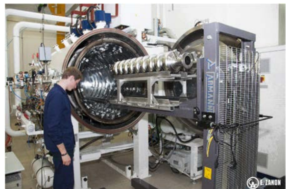
FIG. 8. Furnace for 800 °C annealing at EZ (courtesy of EZ).
