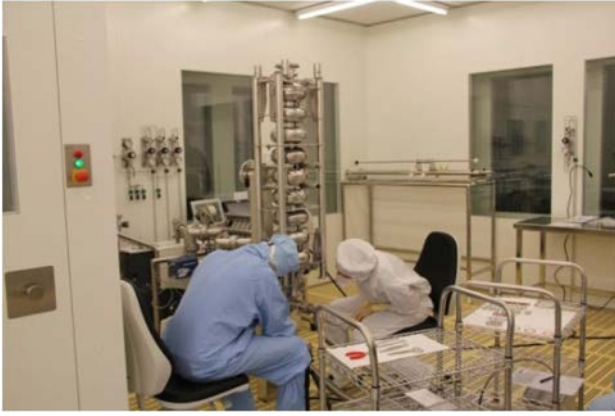
FIG. 5. Flange assembly in the ISO 4 clean room at RI (courtesy of RI).
