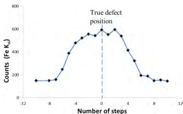
FIG. 9. Line intensity of K_{\alpha} peak of iron as a function of lateral displacement of the sample with 0.5 mm steps. Step 0 corresponds to the true defect-position.
