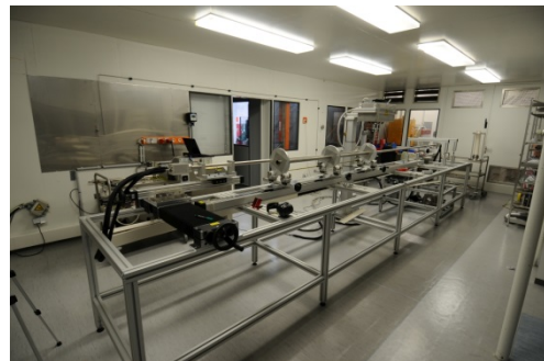
Figure 5: Entire new Installation with mounted dummy pipe.
