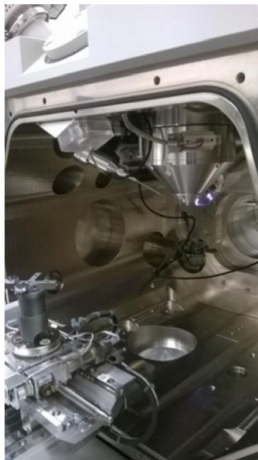
Figure 3: Chamber-view inside the SEM with pole shoe, gas injection needle and sample table. IR-CCD camera permits to track the sample position.
