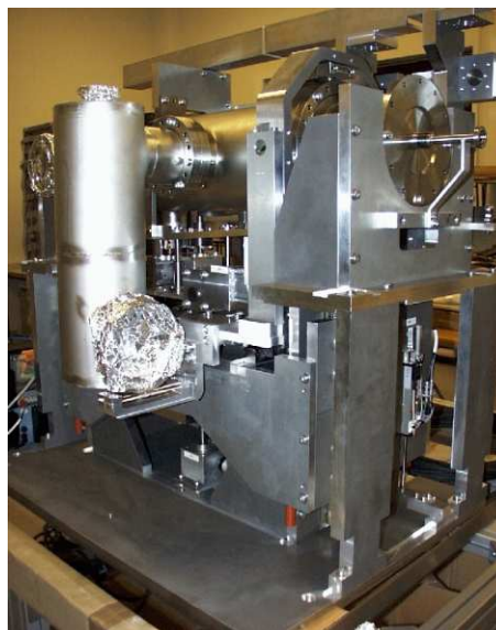
Figure 3: Vacuum chamber of the BTM prototype mounted onto its precise adjustment table.
