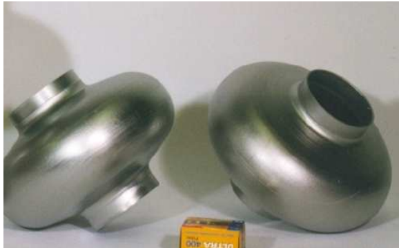
Figure 1: Mono cell cavities fabricated at DESY.
