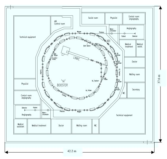
Figure 1: Layout of the angiography facility
