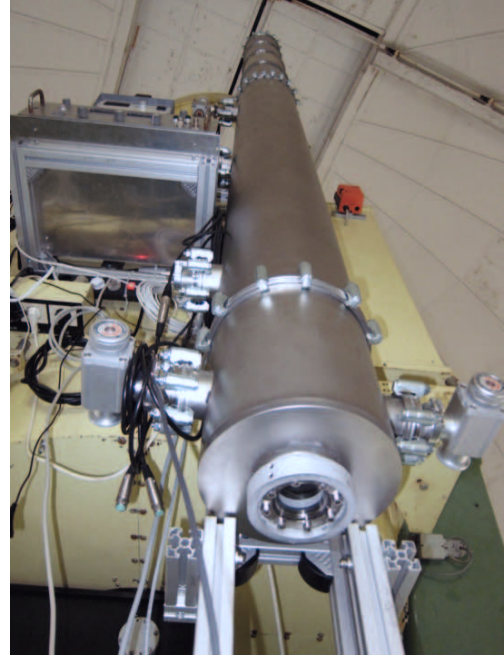
Figure 1: The helioscope TSHIPS attached to the equatorial mount of the Oskar Lühning Telescope at the Hamburger Sternwarte.
