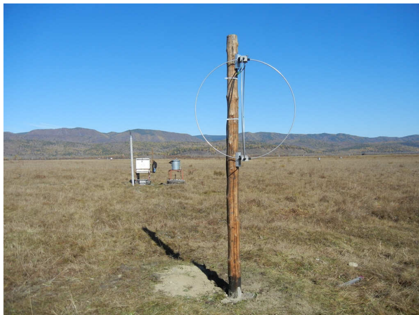
Figure 2. A Tunka-Rex antenna station with its two perpendicularly aligned SALLA antennas.
