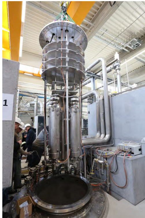
Fig. 4. Installation of the vertical insert into the cryostat.
