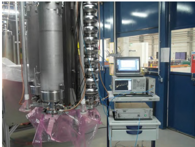
Fig. 3. Setup for vacuum connection and rejection filter tuning.
