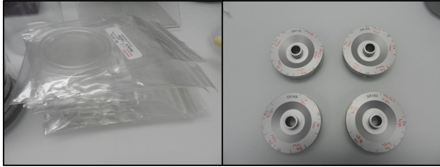
Figure 2.16: Single-element standards from nanoXRF (Fort Worth, TX, USA). (left) Produced as standards of 47 mm in diameter. (right) Strip of standard mounted on RDI wheels to analyse with SR-XRF.
