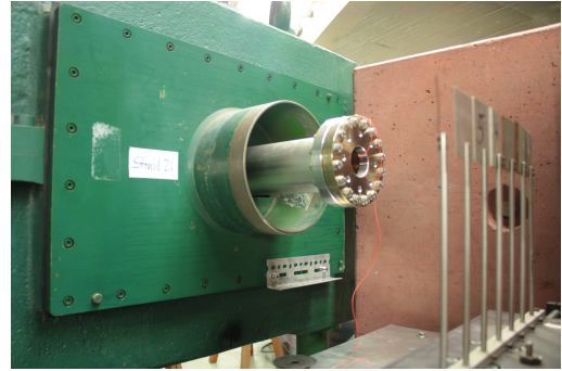
Figure 5.15.: Picture of the different converter plates of test beam line 21 in front of the bending dipole magnet. The aluminium beam pipe is evacuated and has a Kapton beam window. The green iron pipe around it belongs to the magnet surrounding and does not serve any special purpose.
