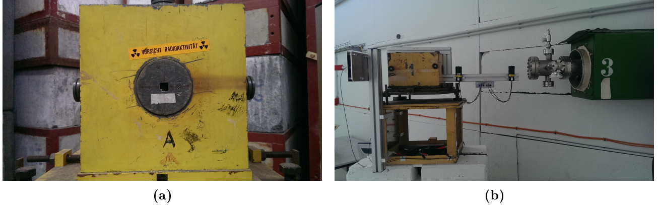
Figure 5.26.: Photos of the collimator in the test beam areas. The beam enters the test beam area through the beam pipe and is collimated by the shown collimator. The user can chose from insertions with holes of different sizes from 2\text{ mm} \times 2\text{ mm} up to 1\text{ cm} \times 1\text{ cm} .
