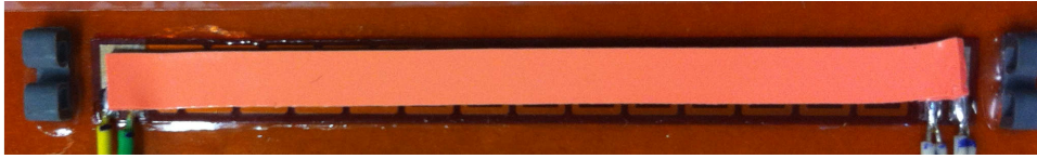
Figure 5.10: The thermally conductive foil does not cover the full heater, due to its smaller width. Measurements might be influenced.
