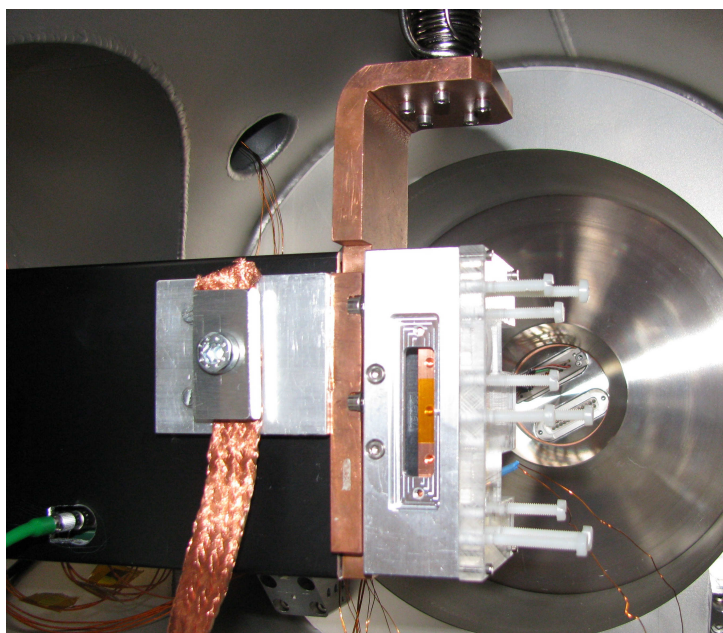
Figure 5. The single chip Germanium system inside a vacuum test chamber. The detector head is connected to a Cryotiger cooler from above. The readout electronics (inside a housing) are connected to power and signal output cables via a connector on the chamber wall. A miniature X-ray tube is mounted in the wall of the chamber (not visible).
