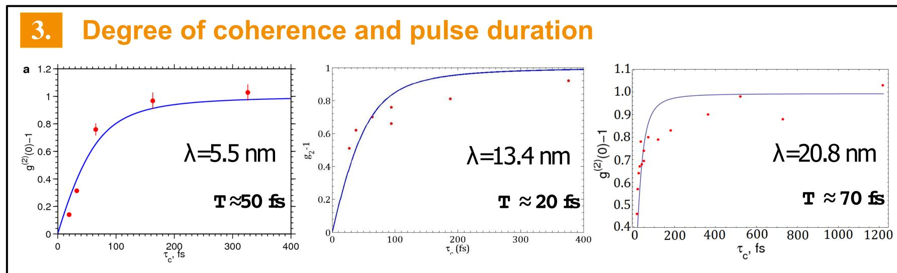
Contrast as a function of coherence time for different wavelengths. Pulse durations: (a)  $T \approx 50$  fs; (b)  $T \approx 20$  fs; (c)  $T \approx 70$  fs. (0.2 nC charge).
