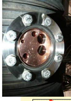
window with new HOM shielding
