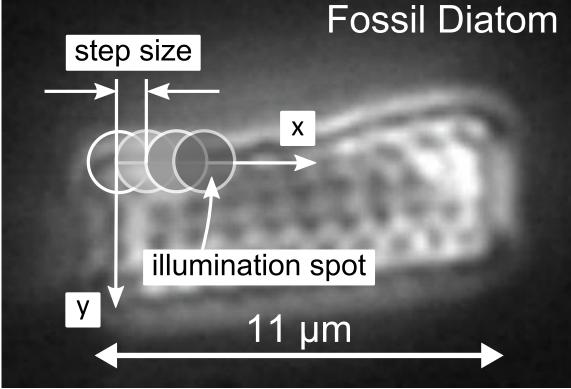
Ptychography is a scaning coherent diffractive imaging method to measure extended objects at high spatial resolution
