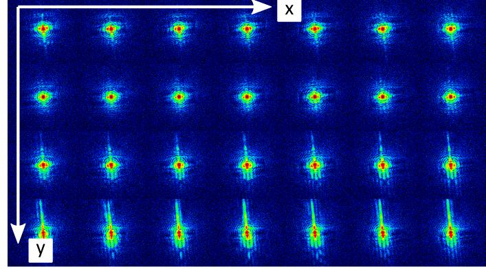
17 horizontal by 7 vertical diffraction patterns (only 7 by 4 patterns are shown here)
