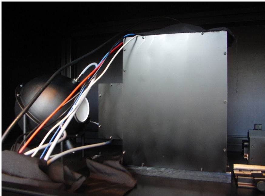
Figure 4. Picture of the setup for PTC measurements. On the left side of the picture the integrating sphere is shown. As a light source an LED is connected to the sphere. On the right side the box containing the camera with its electronics is shown.
