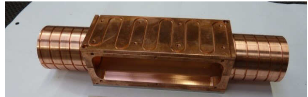
Figure 3: Copper heat conducting elements.
