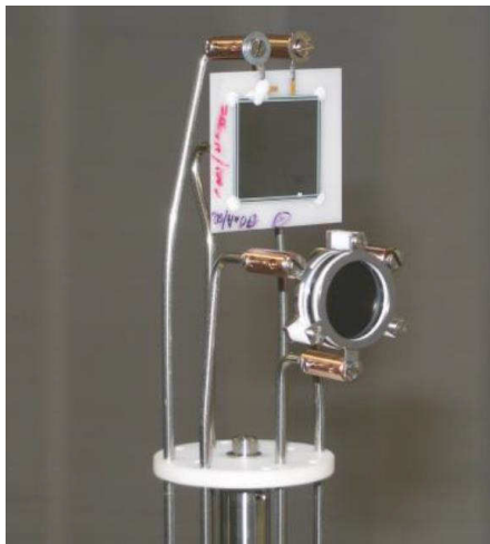
Figure 2: Silicon photodiode and MCP F4655 in the MCP detector prototype.
