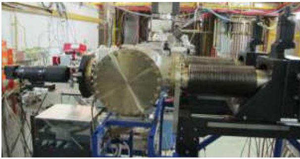
Figure 1: View of SASE1 and SASE2 MCP detector during the DORIS test validation.
