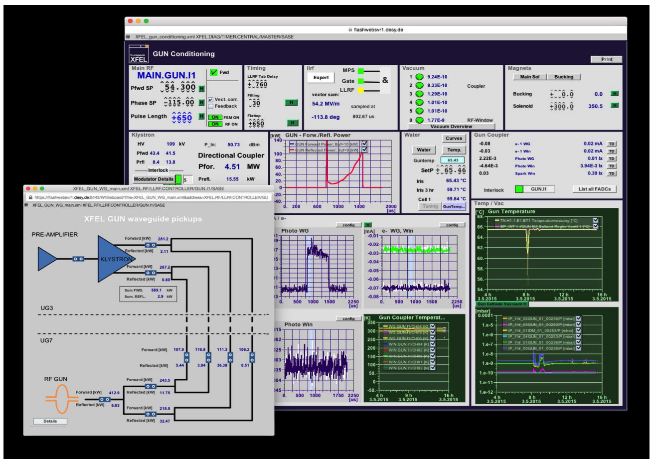
Figure 3: Screenshots of the JDDD web interface running in a Safari web browser (bigger panel) and in a Firefox (smaller panel). All useless browser toolbars are removed and each panel is opened in a separated window. Thus the look and feel and the operation of the panels is equivalent to native JDDD.
