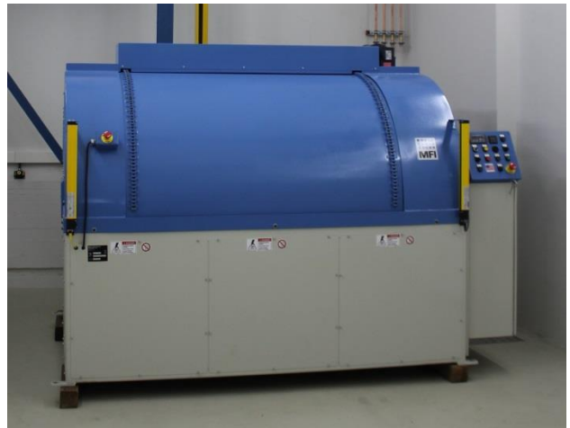
Figure 5: Centrifugal Barrel Polishing machine in the ILC-HiGrade Lab.
