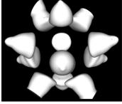
FIG. 8. Isosurface plots of electron densities about the  $B_{12}$  cluster. Left: in  $\alpha$ - $B_{12}$ ; right: in  $\gamma$ - $B_{28}$ . The plotted surface corresponds to the density of 0.84 electron Å $^{-3}$ . They demonstrate the proposed orbital order by lobes of high densities perpendicular to the surfaces of the clusters.
