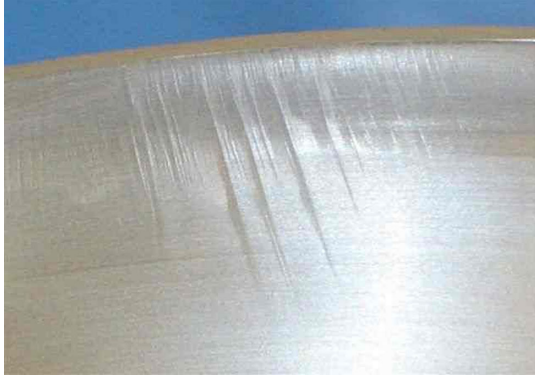
FIG. 18. Slip lines of the crystal on a half-cell after deep drawing.
