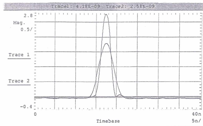
Figure 1: Bunch display just before bunch rotation (Trace 1) and the same bunch at extraction time (Trace 2).
