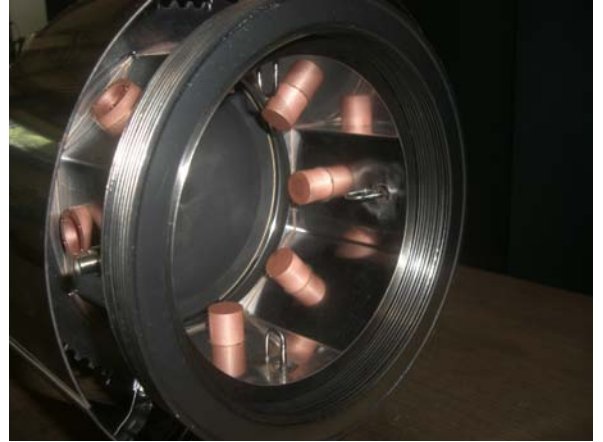
Figure 5: The end of the diagnostics beam line with the wire-loops. The 8 cylinders upstream of the wire loops contain beam halo monitors [1].
