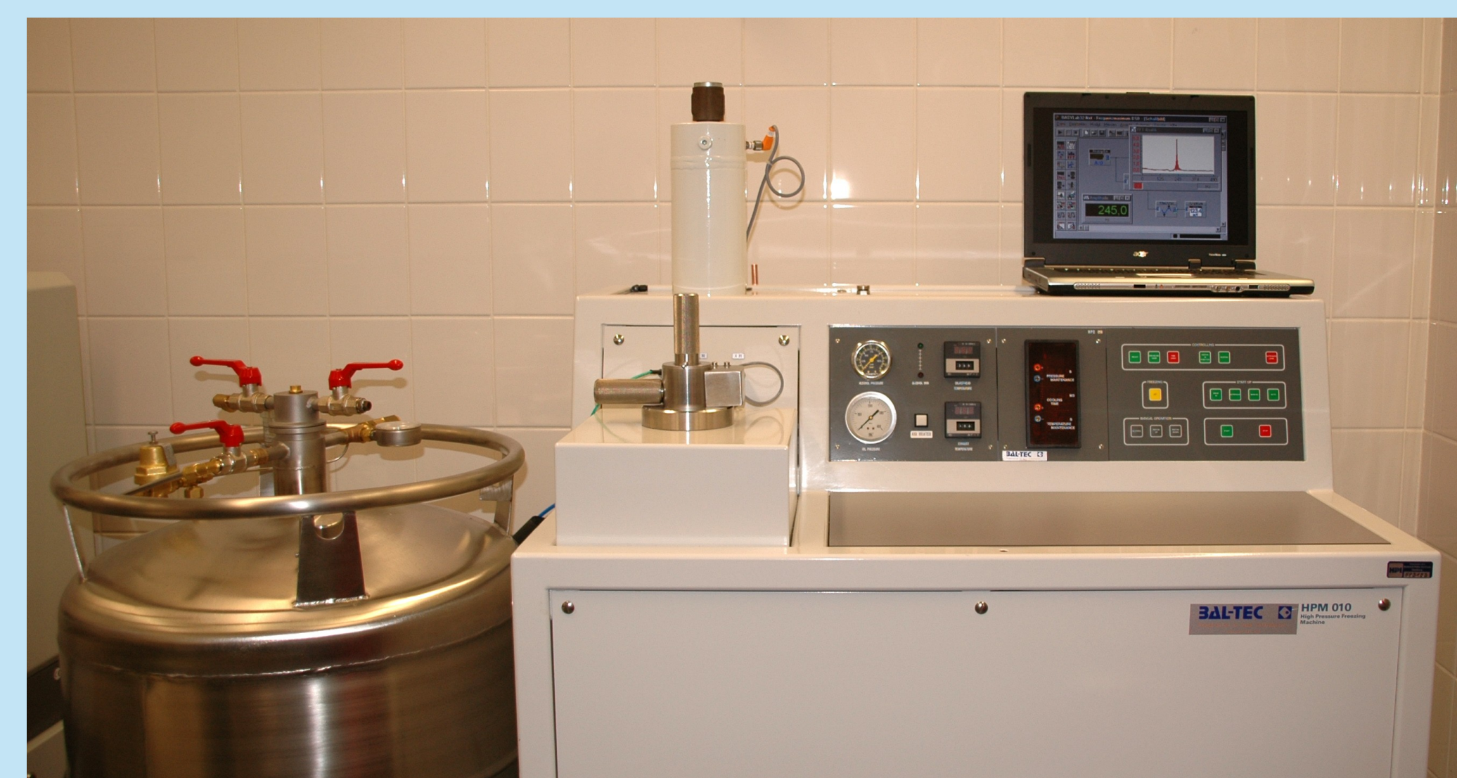
Bal-Tec HPM 010 high-pressure cooling device.
