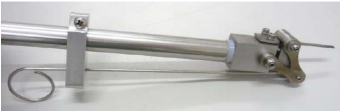
Figure 21 – Device used for testing the shape memory effect
