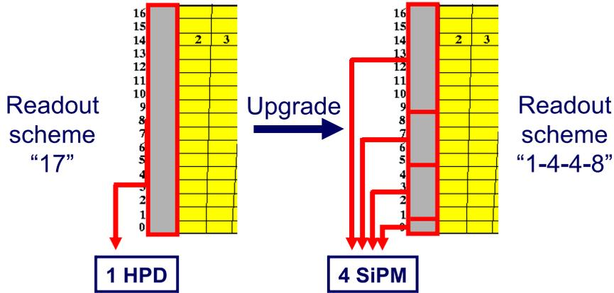
**Figure 4.1:** Schematic illustration of the HCAL readout before and after the Phase II upgrade. Here, the possible readout scheme “1-4-4-8” is shown. The currently used hybrid photodiodes (HPDs) will be replaced by silicon photo multipliers (SiPM).
