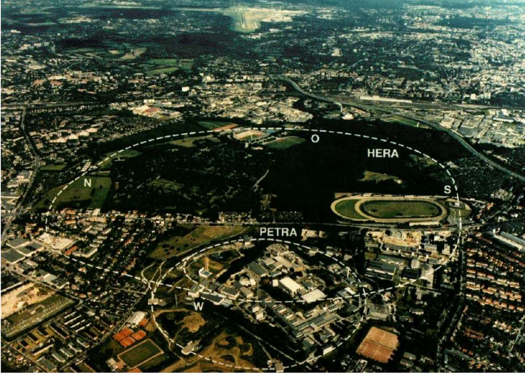
**Figure 3.1:** Aerial view of the DESY laboratory in Hamburg. The HERA collider is marked with the dashed line. In addition the pre-accelerator PETRA (enclosing the main DESY site) is shown in the foreground. The ZEUS detector was situated off the main DESY campus at the south side of HERA.
