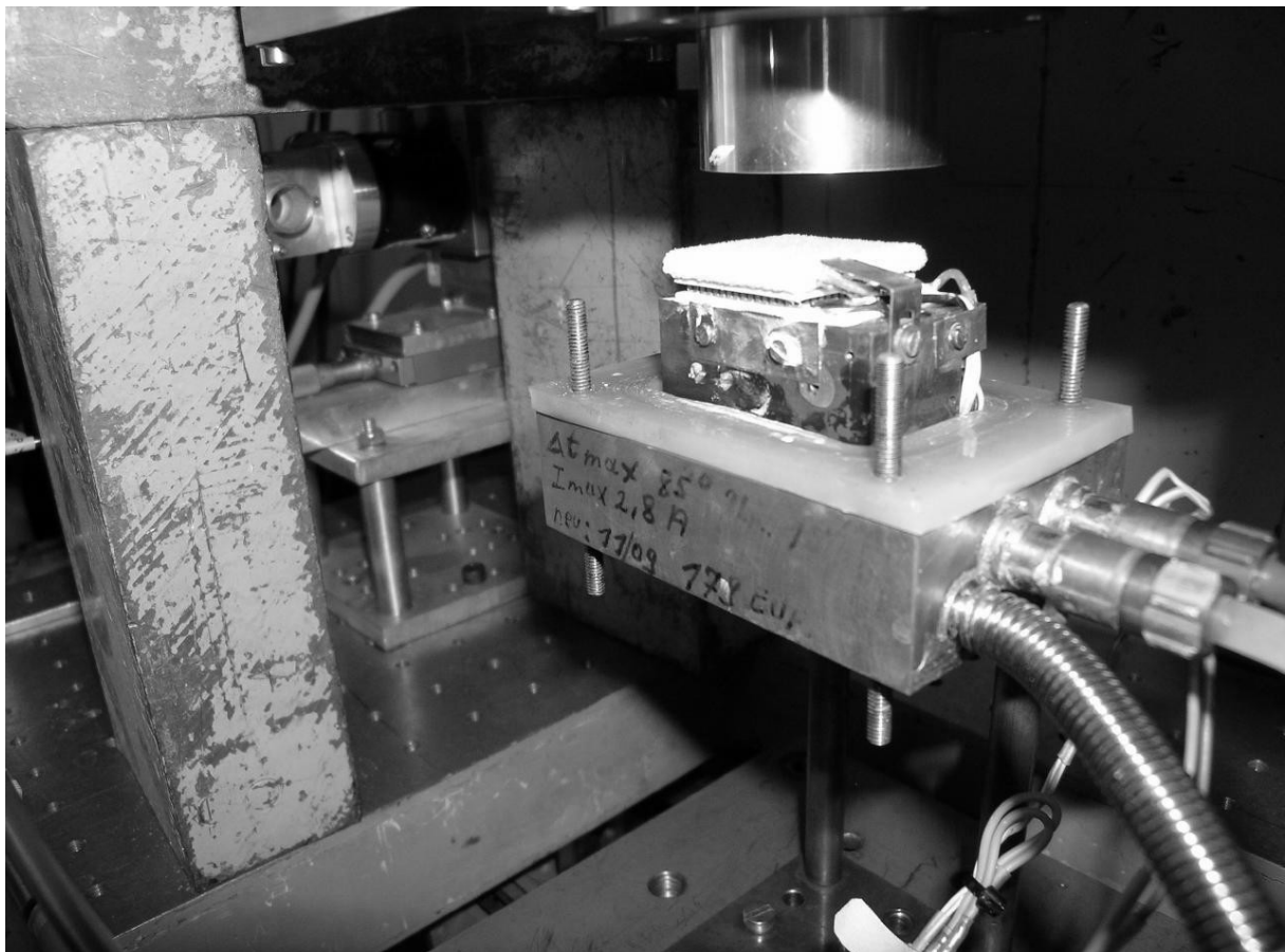
Fig. 1: Set-up for energy dispersive diffraction imaging on frost in transmission mode. The beam enters from the left through a slit system. The capillary optics is located in the cylinder above the specimen which is produced by exposing a two stage Peltier cooler to air.
