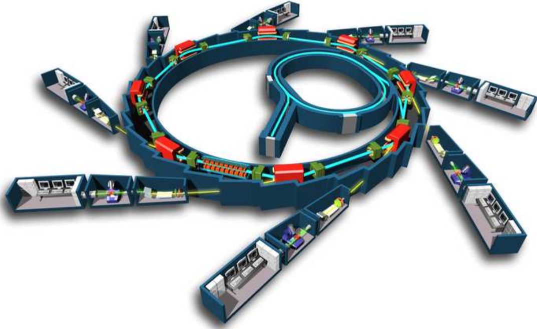
Figure 2.8: Schematic representation of a typical synchrotron, storage ring and associated facilities (pictured is the Soleil synchrotron of Paris, France). An electron gun produces an electron beam which is injected into a booster ring accelerating the electrons further. Periodically electrons from this booster ring will be inserted into the storage ring that produces the synchrotron radiation at the bending magnets and insertion devices making it available for experiments. Source: http://www.synchrotron-soleil.fr/
