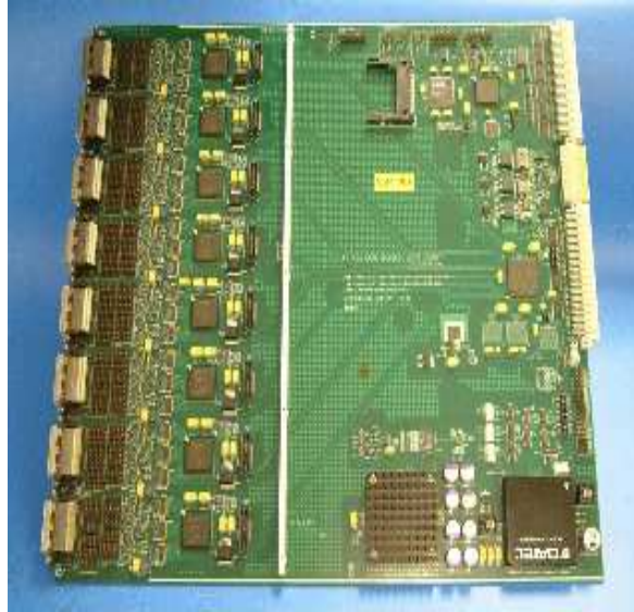
Figure 7.8: CALICE Readout Card. From [269].
