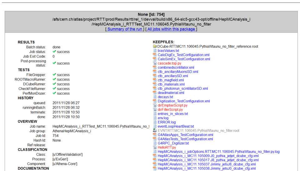
Figure 6.8: Screenshot of a part of the RTT homepage [198]. Results of one of these test jobs for pp \rightarrow W \rightarrow \tau\nu_\tau events of the MC generator PYTHIA6. A list of many files is shown. A graphical visualisation of this test job is done via the DCube Service [199, 200].
