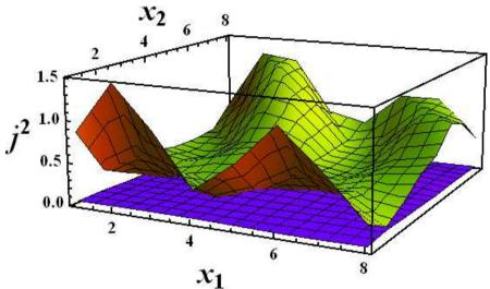
The squared components of the electric current in a 12-plane. The upper sheet represents the spatial distribution of the longitudinal current, the lower sheet corresponds to the transverse current.
