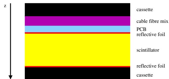
Figure 4.2: Profile of an AHCAL readout module.
