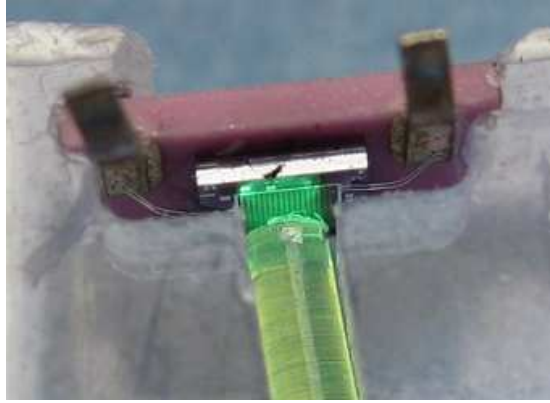
Figure 4.4: Example of a not fully centred light cone on the SiPM surface.
