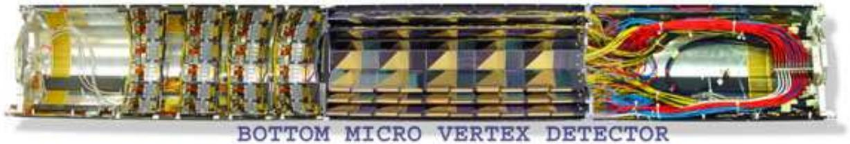
Figure 3.8: The bottom half of the MVD showing the ladders in the barrel, the forward wheels with silicon sensors on the left and the readout cables and services on the right.
