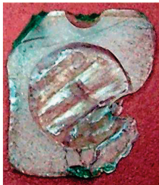
Figure 1. HEPP film after a melting and recrystallization experiment. Aluminum foils are removed.
