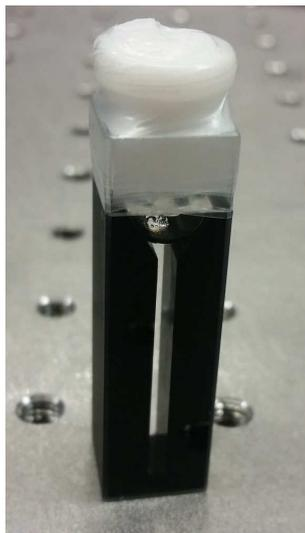
Figure 3.4: Sample cuvette from Thorlabs GmbH [8] with Parafilm<sup>®</sup> sealing
