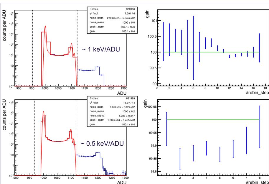
A test of the global fit function was performed with rebinned, simulated spectra resembling the situation of the coarse 8-bit binning of the DSSC. The fit can only be performed by fixing certain parameters. During the rebinning, the offset was changed incrementally (#rebin\_step). The accuracy of the gain determination (green line refers to the theoretical value) needs to be better than the setting granularity of 2%.
