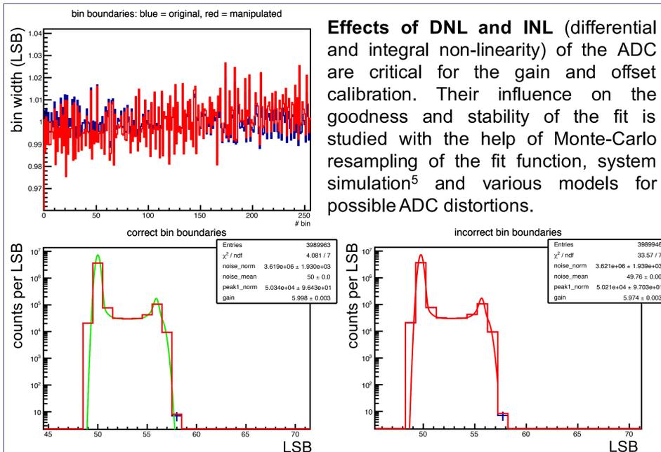
Effects of DNL and INL (differential and integral non-linearity) of the ADC are critical for the gain and offset calibration. Their influence on the goodness and stability of the fit is studied with the help of Monte-Carlo resampling of the fit function, system simulation<sup>5</sup> and various models for possible ADC distortions.
