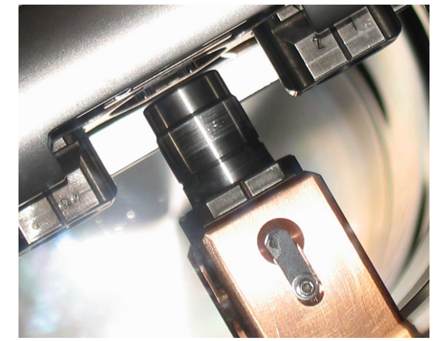
Cathode plug extracted from the carrier.
