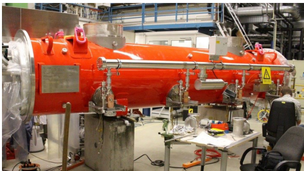
Figure 11: The 3.9 GHz harmonic module during its final preparation stages before installation in the E-XFEL injector tunnel.
